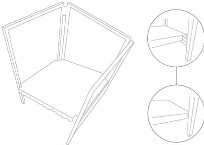
Starting at the bottom, gently slide each shelf into position. Ensure the shelf is slotted into place and secure before moving on to the next.
