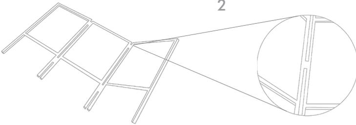
Lie the frame on a flat surface to open and stand the frame so this is in square form. Assemble in desired situ to avoid carrying.
